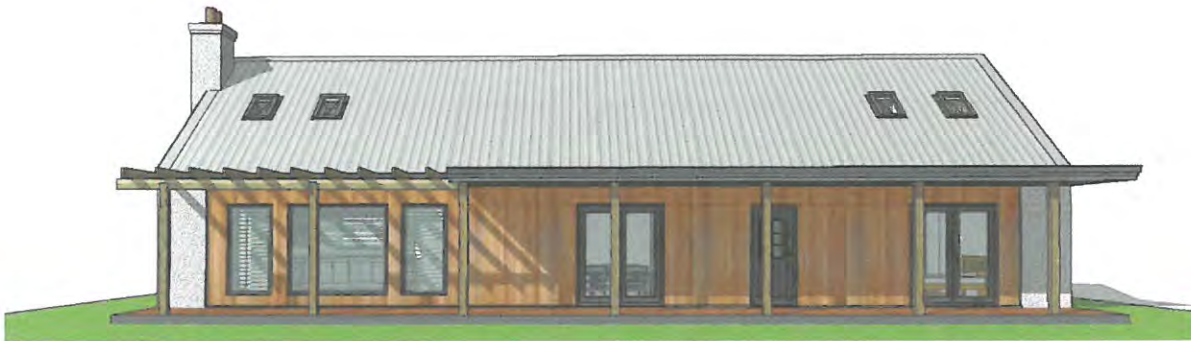
The South Elevation to the rear – opened up to light while providing summer shading with planted pergola and projecting roof
