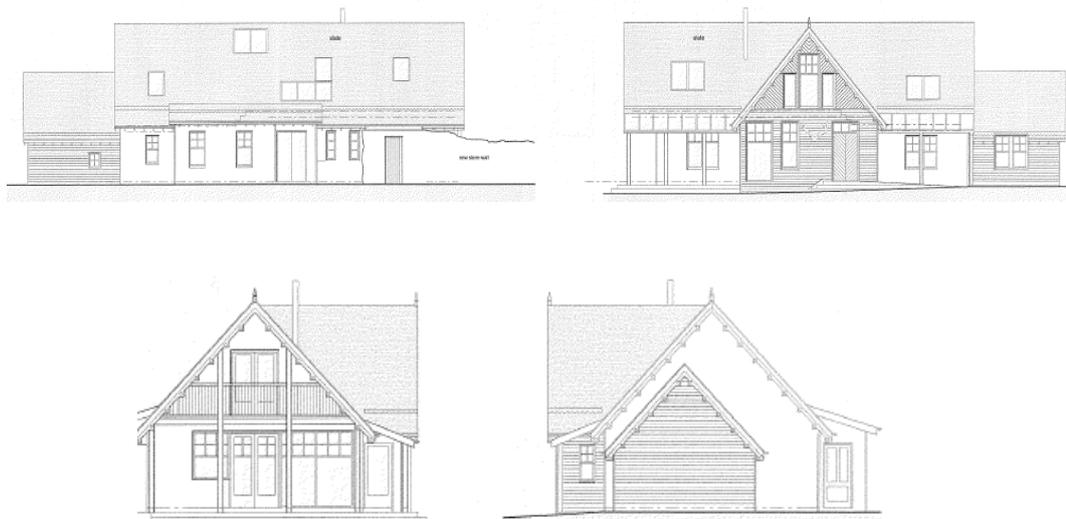
**Fig. 8 - New elevations (changes: smooth render and slate)**
